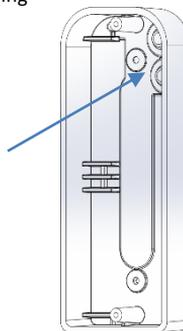
5. Replace the metric screw with those present in the bag and insert the seals in the compartments as indicated
