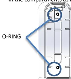
6. Screw the transmitter holder to the plate
