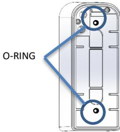
8. Drill the concentric seal and pass through the tamper cable
