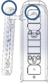
14. Secure the NAT base with the screw located at the bottom
