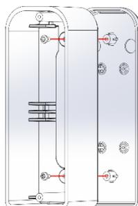
7. Check that the seals in the canopy are inserted correctly
