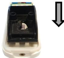
3. The device can be removed by levering with the screwdriver underneath.
