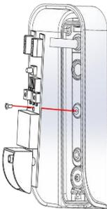
12. After performing the calibration, insert the sensor cover and close everything with the screw located under it
