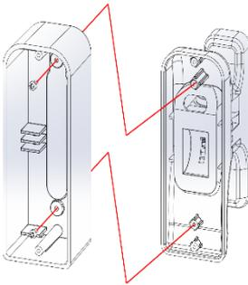
10. Check that the canopy seals are inserted correctly
