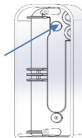
7. Replace the metric screw with those present in the bag and insert the seals in the compartments as indicated
