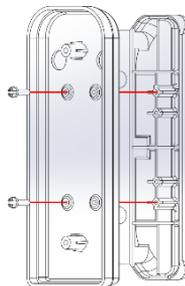
3. Remove the metal plate from the back of the transmitter holder
