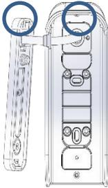
10. Secure the NAT base with the screw located at the bottom
