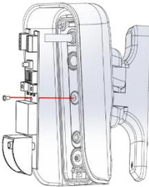
16. After performing the calibration, insert the sensor cover and close everything with the screw located under it
