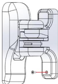
4. Adjust the inclination (from 0° to -30°) and the horizontal rotation (180°) and fix everything with the central screw
