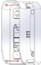
6. Make a hole in the concentric seal to allow the passage of the cable and insert it into the NAT base
