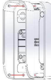
9. Make a hole in the seal to allow the passage of the cable and insert it into the NAT base. Insert the hook of the Nat base in the canopy compartment as shown
