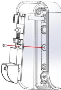
10. After performing the calibration, insert the sensor cover and close everything with the screw located under it
