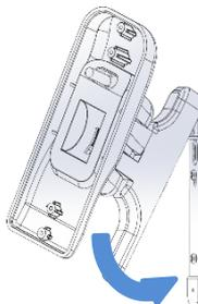
3. Tighten the screw located at the bottom
